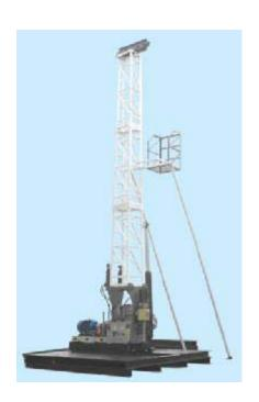
drilling vertical as well as inclined holes. The range of adjusting angels (in clock-wise direction) for drilling inclined holes is  $0^{\circ}$ - $90^{\circ}$ .
